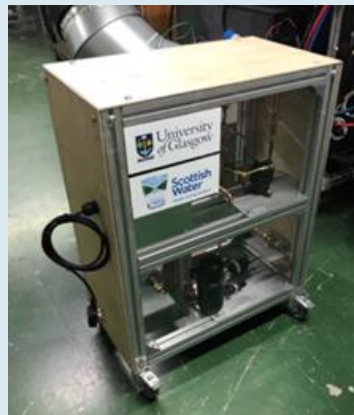
Fig 1: Integration of heat pump and biofiltration unit: A) schematic B) Heat Pump C) Biofilter unit integrated into heat pump.
